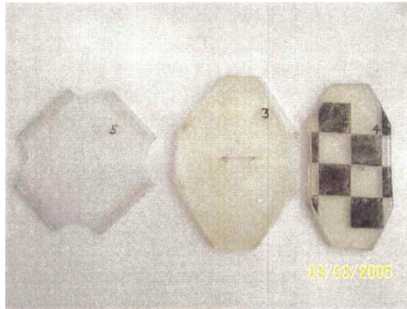
Figure 34: Samples with Increasing Prestrain, From Left to Right (0%, 28%, 60%) Recovered to Their Original Shape after Testing
