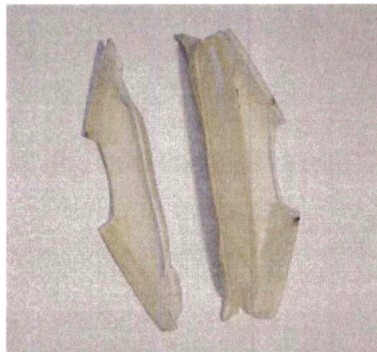
Figure 38: Specimen 2 Fractured from Compression
