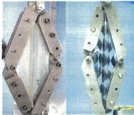
Figure 31: Samples #2 and #1 Showing Folding of SMP During Testing
