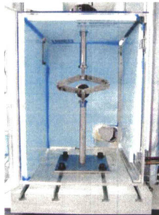
Figure 22: Shear Fixture (Without Specimen), Setup to Run Diamond to Square Shear Test
