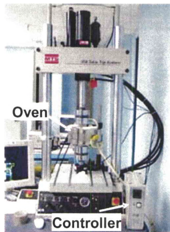
Figure 18: Load Frame Setup for Tensile Testing
