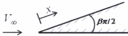
Figure 2.3: Image showing the freestream velocity, wedge half angle and the orientation of the axis.
