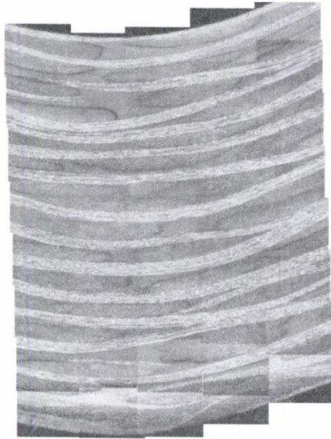
Figure 58. Photomicrograph of 0.25"-Radius 16-Ply Bracket Without NMR Before Applied Load
