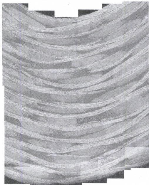
Figure 50. Photomicrograph of 0.125"-Radius 16-Ply Bracket Without NMR Before Applied Load
