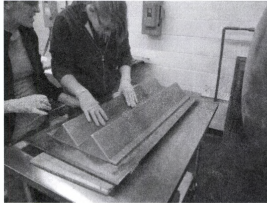
Figure 3. Layup of Composite Angle Bracket Panel
