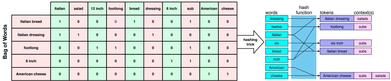
Figure 8: Data structure representation of our bag-of-words model.
