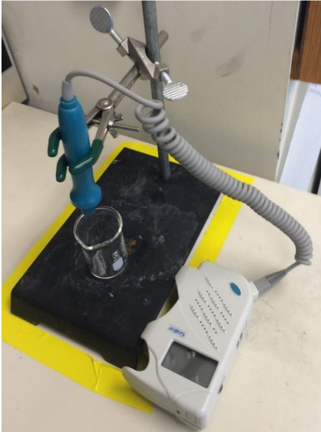
Figure 9: Ultrasound set up. All treatments and trials occurred in accordance with this protocol. The setup is shown in figure. Samples were transferred from their food vials to the beaker. The Grafcop Pocket Doppler emits a 4 MHz frequency and 1.72°C per minute. The setup remain in the same place for all trials to remove factors that could affect the treatments. The height of the probe remained at 10 mm for all trails for consistency.
