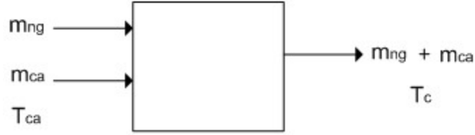
Figure 2. Mass balance on combustion chamber
