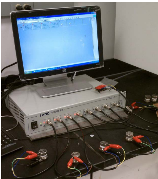
Figure 32: Lithium-ion battery testing system.
