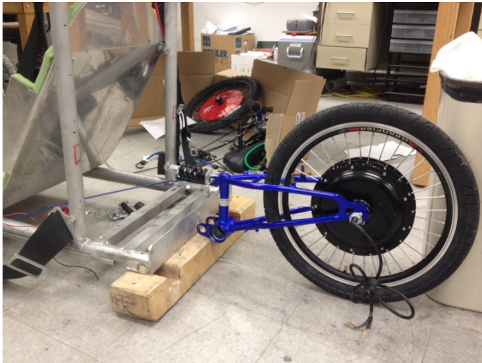
Figure 34: Wheel, electric motor, and rear swing arm for the Wright State eco car.
