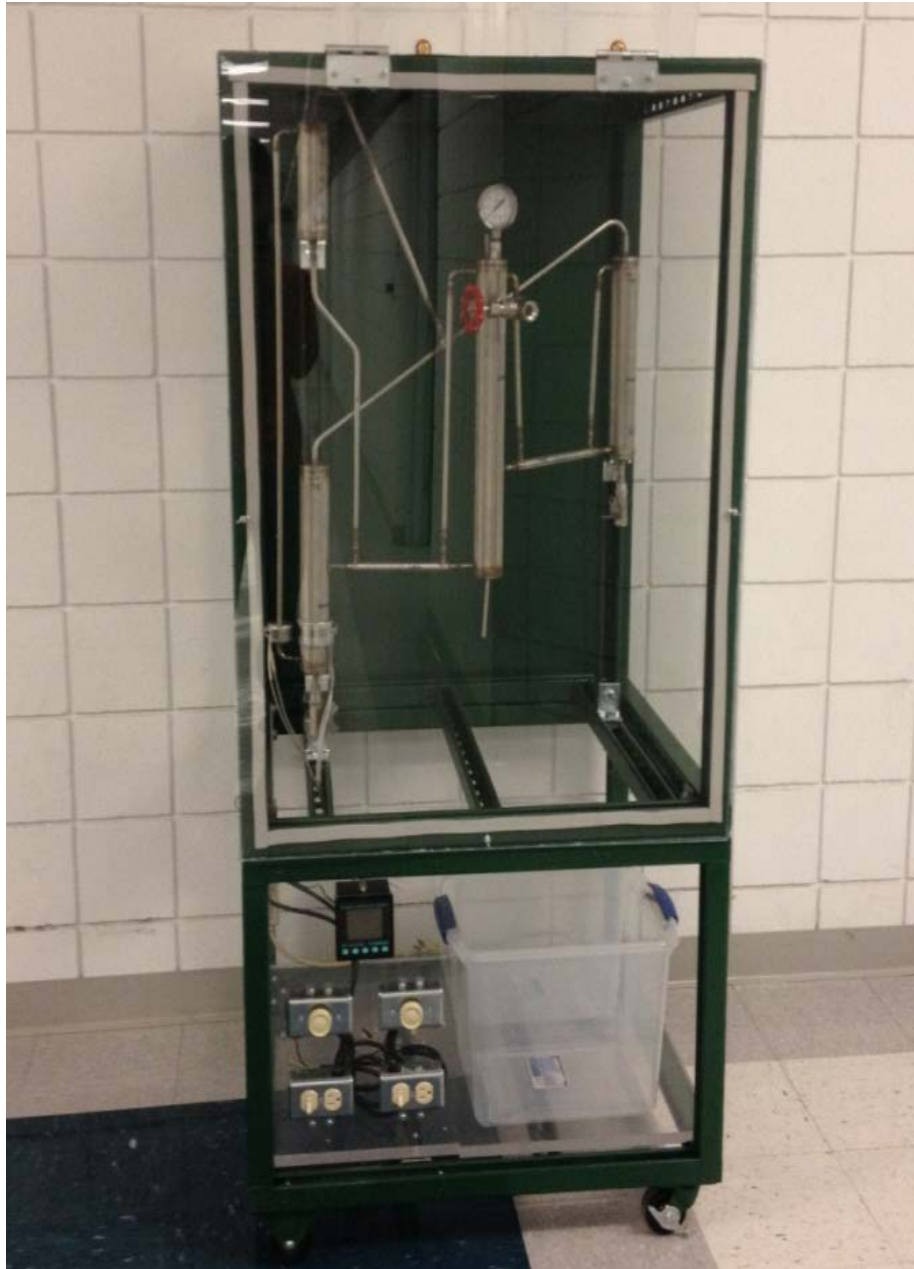
Figure 30: Absorption refrigeration system.
