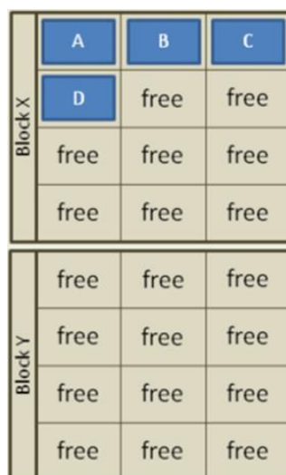
Figure 6: Blocks in solid state drives (Structure of SSD block , 2015)
