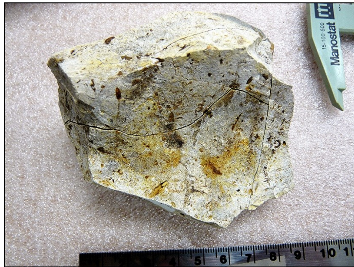
Figure 10. Core comprised of weathered, chalky Pennsylvanian material.
