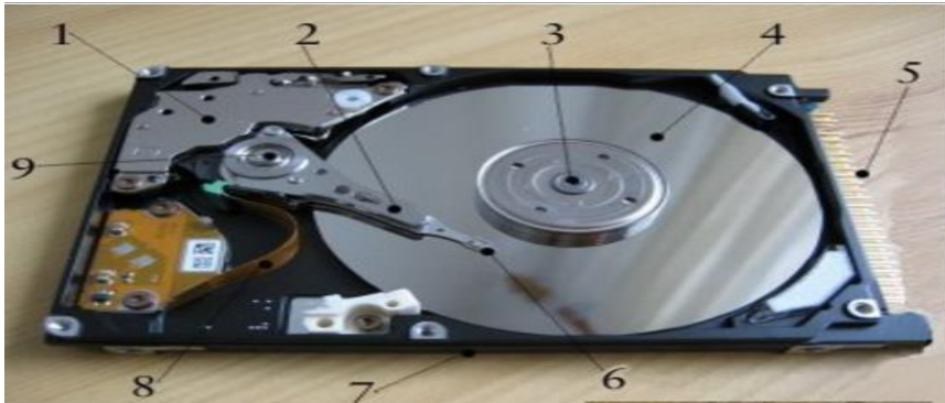
Figure 2. Hard Drive Components (Woodford, 2015)
