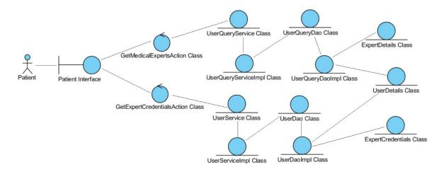
Figure 30: Interaction of classes for the realization of the 'View Medical Expert Information' use
