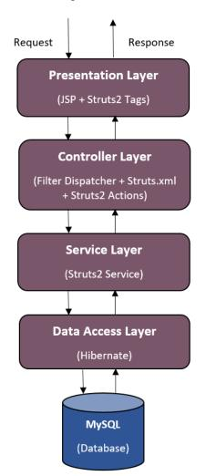
Figure 57: Architecture of Remote Health Service System
