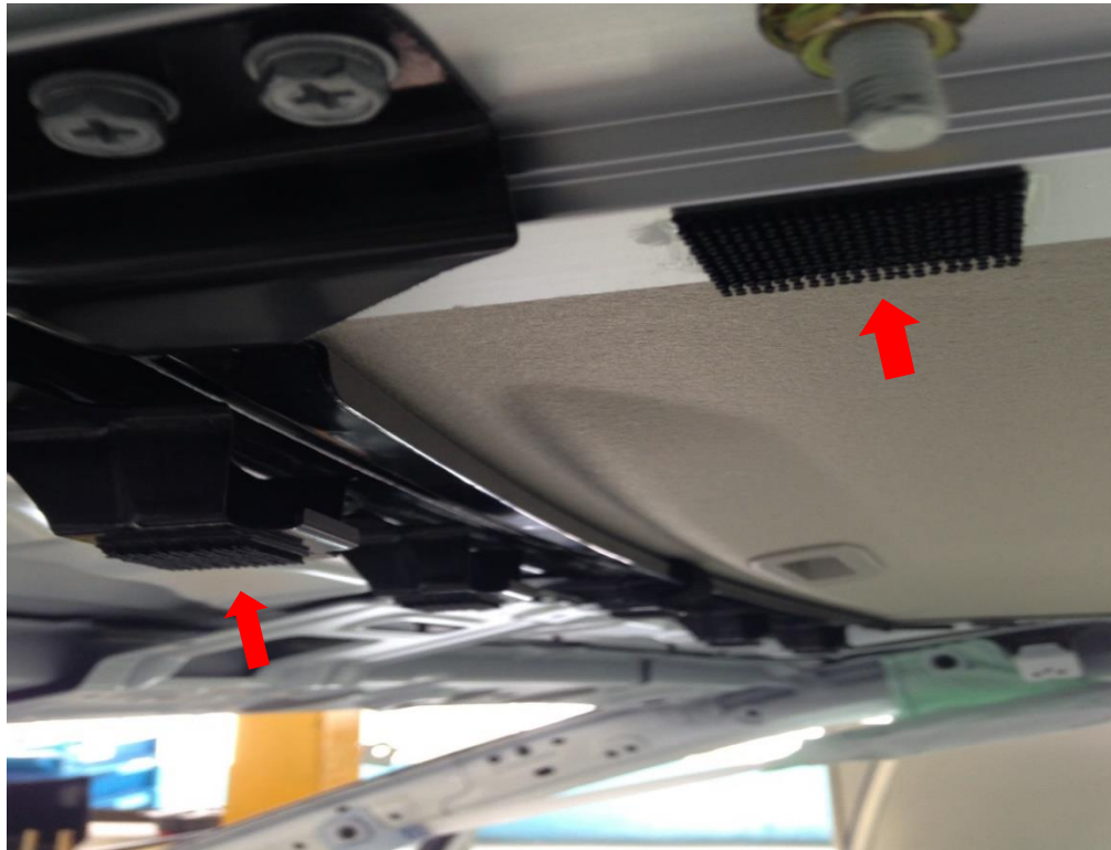
Figure 20: Connected Hasps on Skylight
