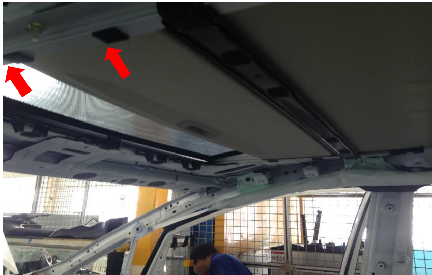
Figure 10: Connected Hasps on Skylight
