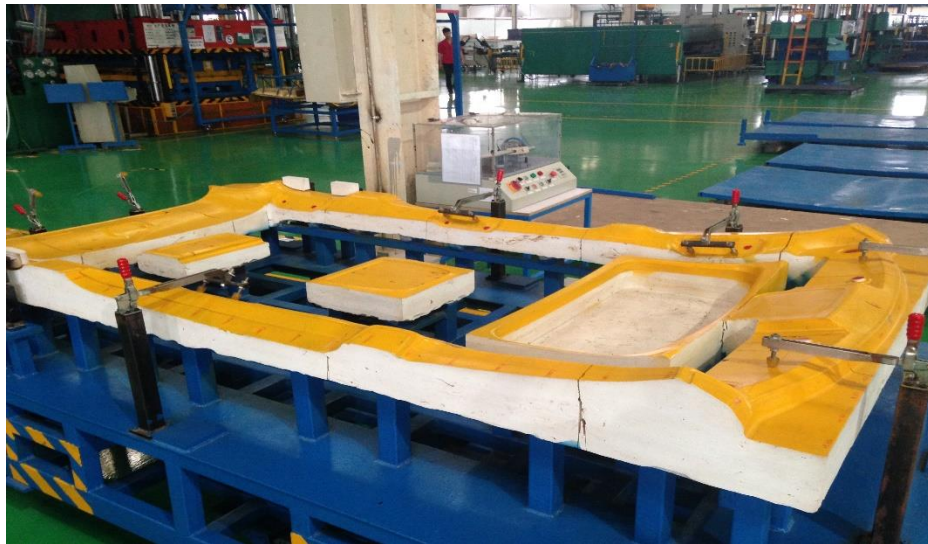
Figure 8: Detection Mold of Plafond
