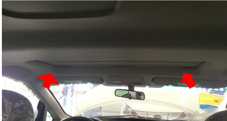
Figure 5: Gap between Skylight and Plafond
