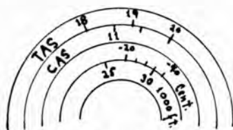
Fig. XII Air speed correction on computer
