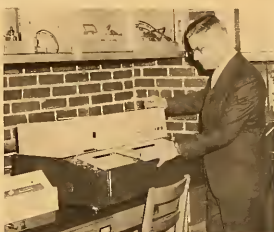
The chemistry department's new Beckman IR-8 Spectrophotometer is adjusted by Dr. John Christensen, chairman of the Natural Science Division. The instrument will be used to identify organic compounds.
