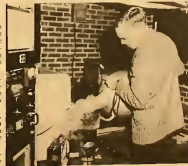
Devising methods to handle and store the cooling agent liquid nitrogen, Mr. William Mundy gears small quantities of the -322 degree liquid. SMC physics research is being facilitated by the use of the liquefied gas.
