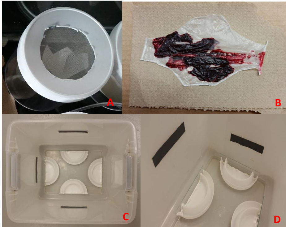
Figure 1. Equipment for containing Bed bugs and testing arena. A- Plastic screw top containers in which Bed bugs; B- Parafilm blood bag; C- Aerial view of testing arena; D- Inside view of testing arena.
