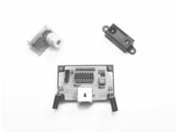
Fig. 7. Some of the sensors currently used with the UP1bot. The digital compass on the upper left is mounted on a PC board designed in-house to interface it directly to the header pins on the UP 1 board. The IR proximity detector with two IR LEDs and one IR receiver is shown on the bottom, and the IR distance detector with offset IR LED and receiver is shown in the upper right.
