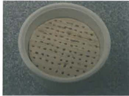
Figure 2. Balsa septum in PVC coupler
