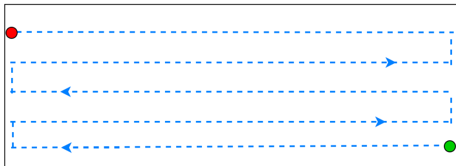
Figure 4.7: Zig-zag motion with sweep direction along the longest edge
