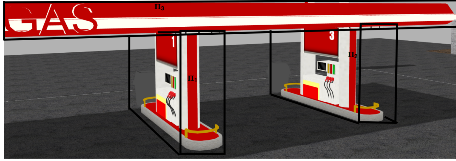
Figure 3.1: A sample target structure of a gas station that needs to be inspected. The solid black lines represent the envelope around the structure
