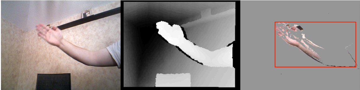
Figure VI.2: From left to right, the RGB image, the depth map (lighter pixels are closer to the sensor), and the background subtracted image with the tracking square.
