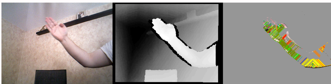
Figure VI.12: (right) The non-edge pixels adopt the the motion vector (and color) of the nearest edge pixel which is on the object boundary within a given radius.
