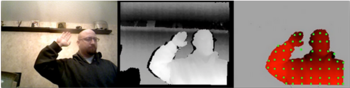
Figure V.5: The calculated centers of mass (shown as green squares) in a real image.
