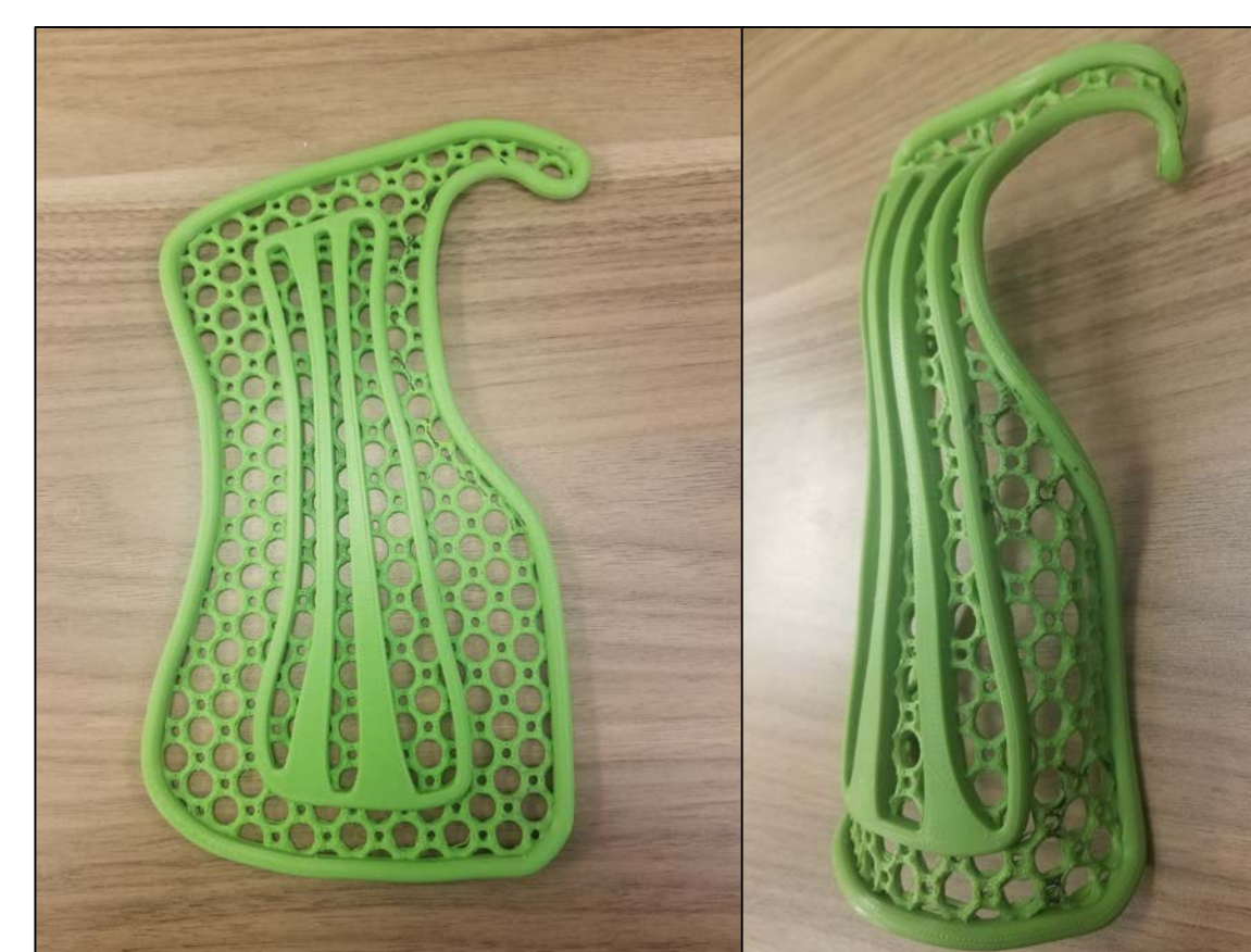
Figure 3: A) Unformed wrist splint; B) A 3D printed wrist splint, thermoformed to fit the user.
