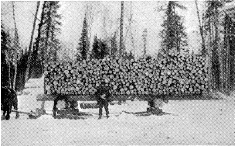
Fig. 36. A Logging Sled equipped with Racks for carrying 8-foot Pulpwood. Minnesota.
