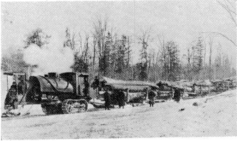
By permission of Lombard Auto T'ractor-Truck Co. Fig. 48. Lombard Steam Log I-hauler.
