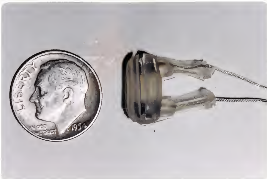
Figure 5. Silastic-shielded, platinum, bipolar electrode used in carotid sinus nerve stimulation.
