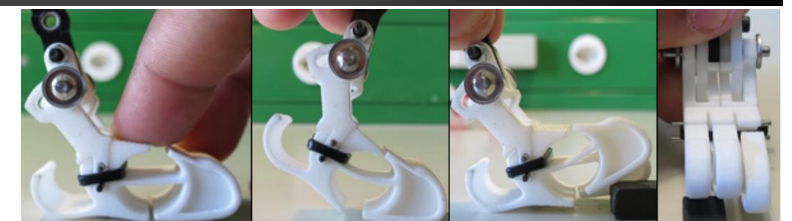
Figure3. Flexible foot prototype performing adaptation to different surface to manually applied force. Adopted from [3].
