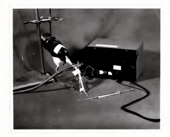
Figure 1: Photograph of rat in restraining holder with pressure cuff, microphone for amplification of arterial pulse, and intravenous needle in place on tail. This is the apparatus used for pressor response measurements.
