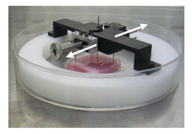
Figure 1. Image of microdistraction model. Note polymerized collagen gel between polyethylene bars and arrows depicting direction of distraction.
