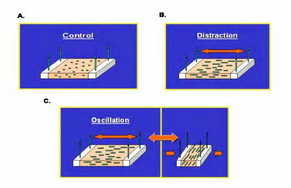
**Figure 2.** Experimental groups. A. Control (no stress applied to gels). B. Distraction (daily lengthening of gels) C. Oscillation (Cycles of distraction and compression).
