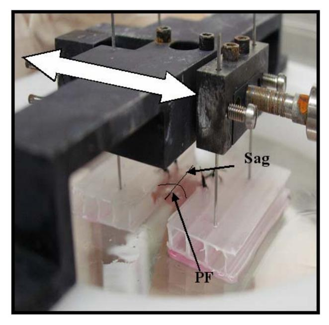
**Figure 2.** Cranial Sutures within Microdistractor: the PF and sagittal sutures are positioned to allow perpendicular stress with activation of the microdistractor.
