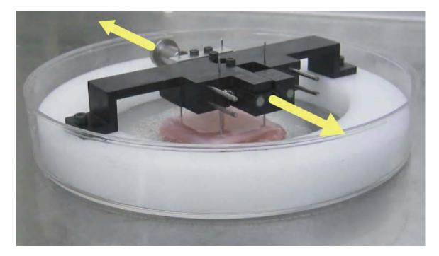
Figure 1. The Microdistractor device with gel in place. Arrows indicate the vector of movement.
