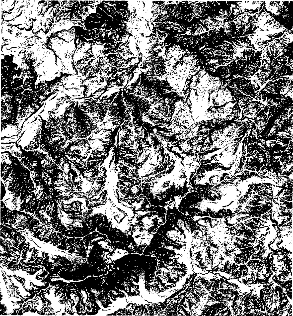
Figure 6: Numerical simulation of the hemispherical shielding of the topography on the diffuse irradiant flux. The average shielding coefficient was calculated for a four kilometer radius around each pixel.
