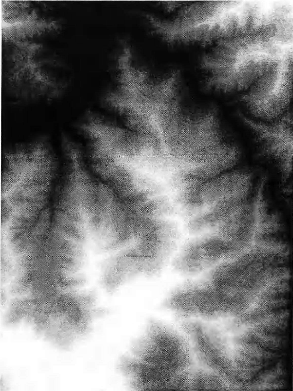
Figure 11: A digital elevation model for a part of Nanga Parbat (Each pixel represents 20 meters by 20 meters).
