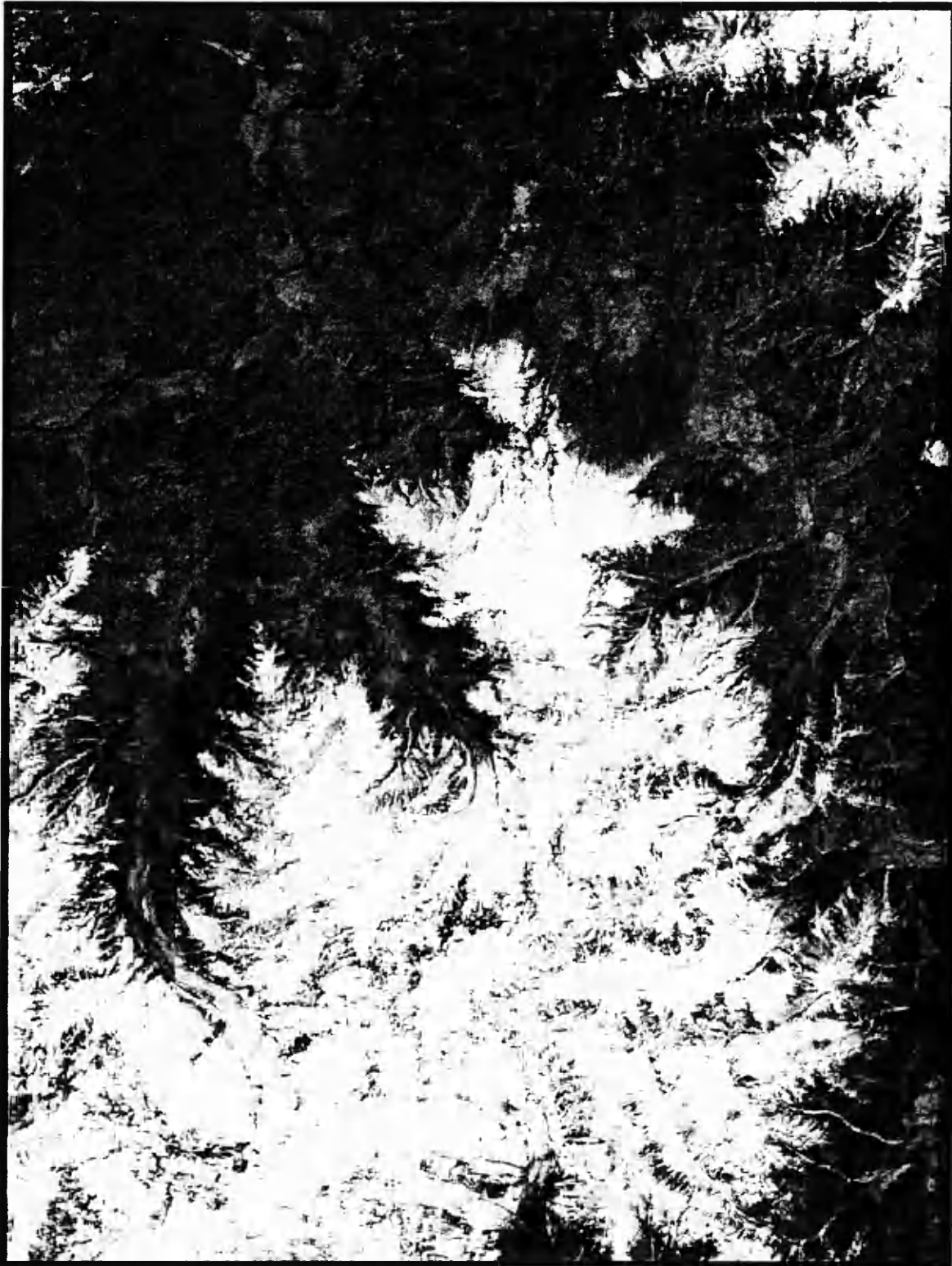
Figure 19: SPOT-3 NIR normalized image using the Minnaert-correction procedure and multiple Minnaert constants based upon window analysis (21x21 pixel window).
