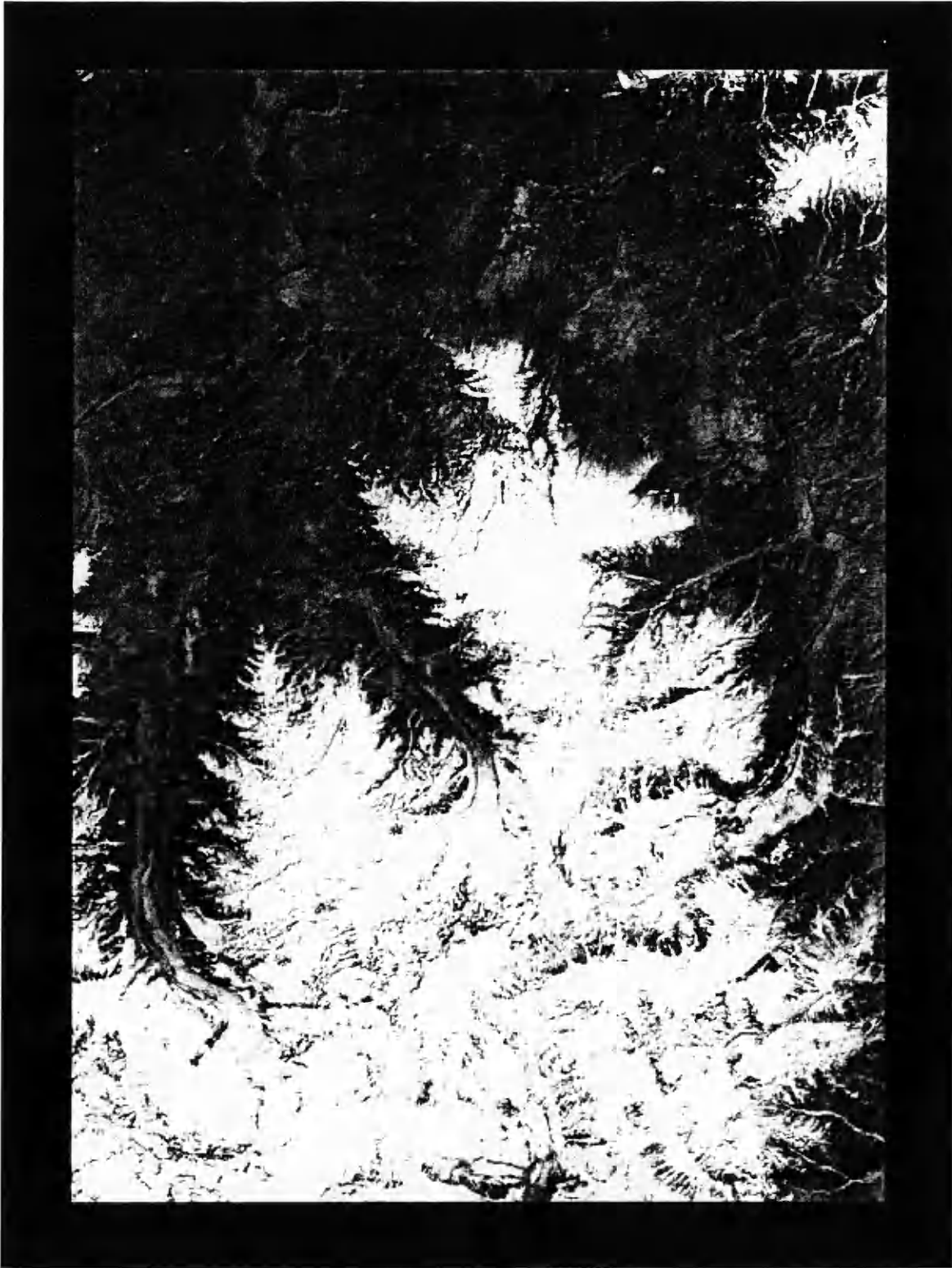
Figure 21: SPOT-3 NIR normalized image using the Minnaert-correction procedure and multiple Minnaert constants based upon window analysis (201x201 pixel window).
