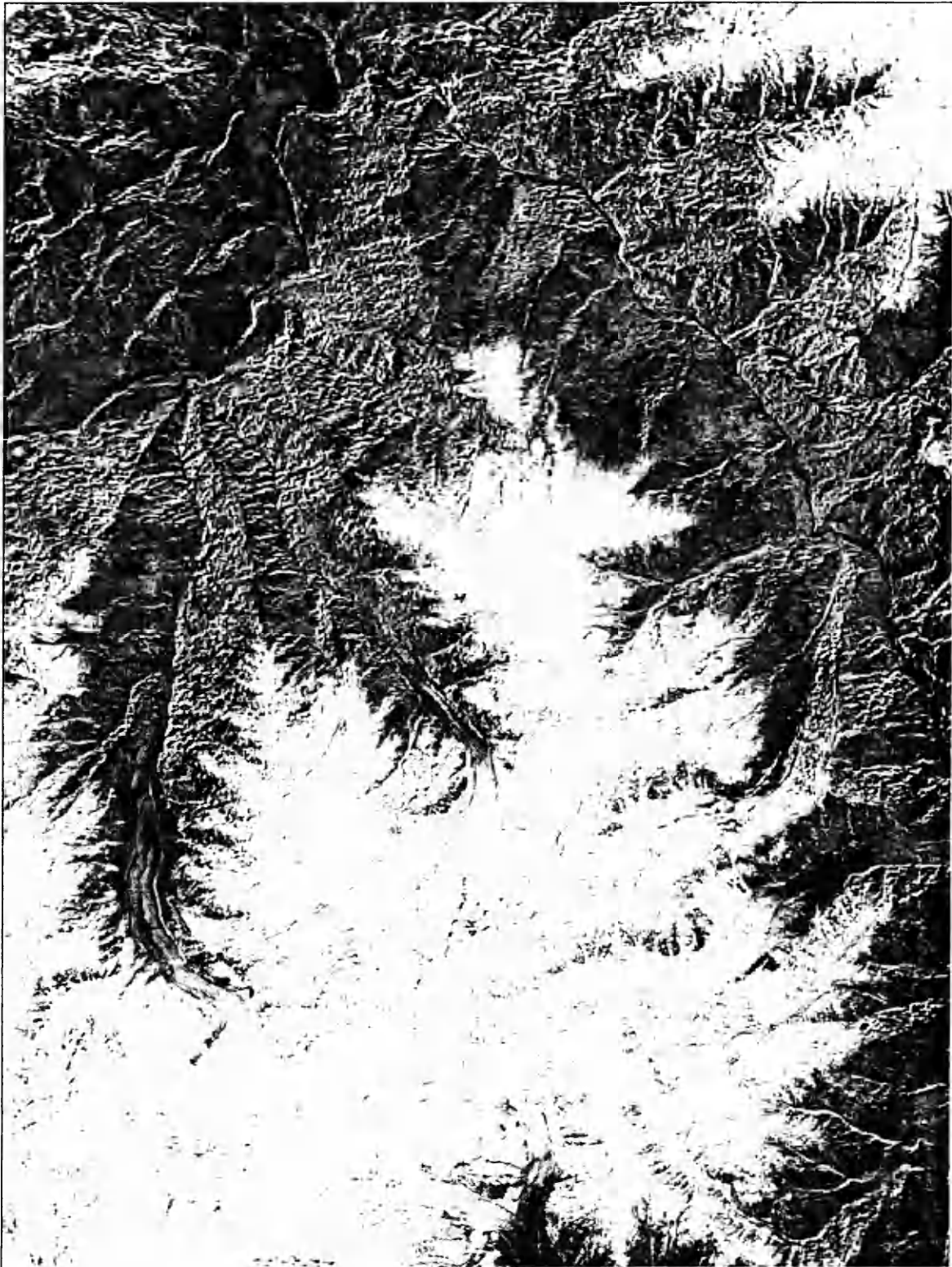
Figure 15: SPOT-3 NIR normalized image using the Cosine-correction method. High radiance values (overcorrection) is the result of steep slopes and relatively low direct solar irradiance.
