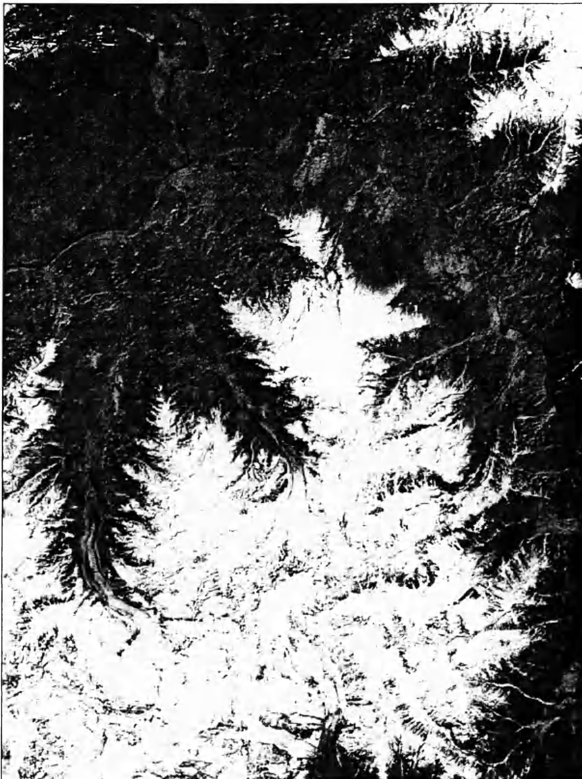
Figure 16: SPOT-3 NIR normalized image using the Minnaert-correction procedure based upon a global Minnaert constant.
