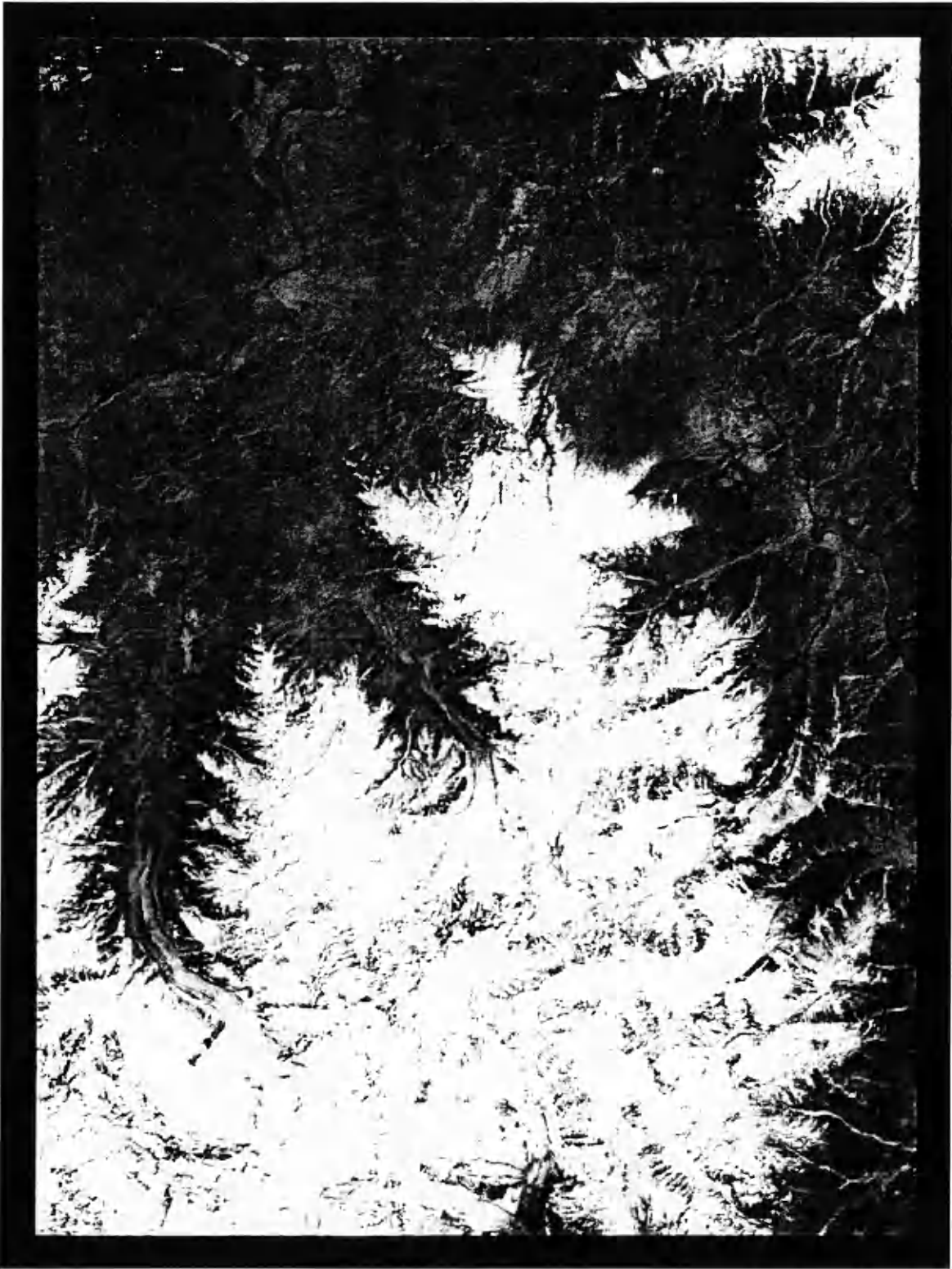
Figure 20: SPOT-3 NIR normalized image using the Minnaert-correction procedure and multiple Minnaert constants based upon window analysis (101x101 pixel window).
