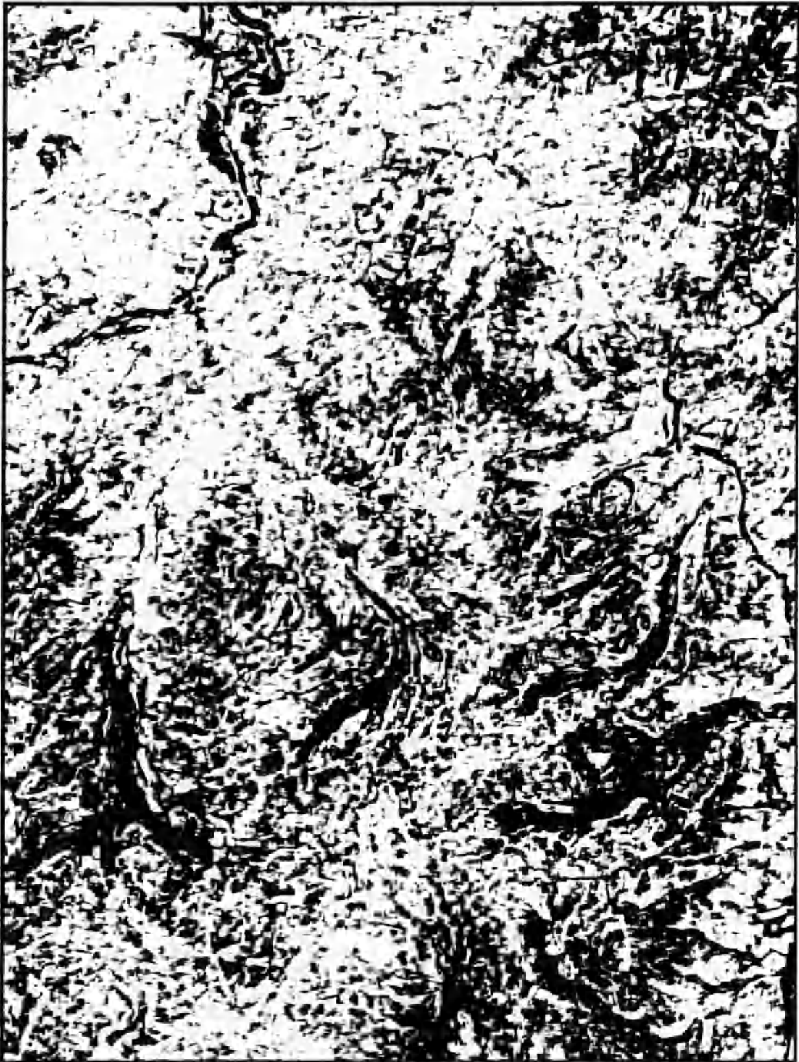
Figure 22: Coefficient of determination ( r^2 ) image based upon regression analysis for a 11 \times 11 pixel window.
