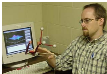
Max Kurz holds a calibration device used for gait data collection .
