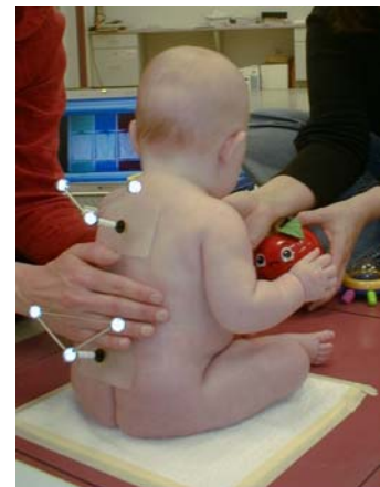
Our typical set up for capturing sitting development on a padded force plate.
