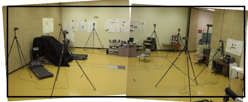
EIGHT-CAMERA MOTION CAPTURE SYSTEM
