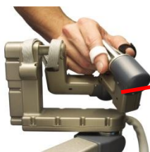
Hand manipulators with eight -degree of freedom motion
