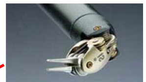
Endowrist® instruments : reproduce hand movements
