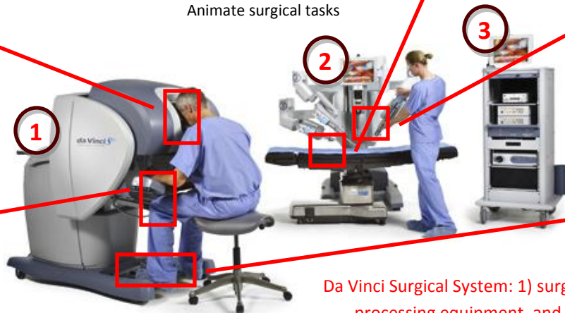
Foot pedals for Dvss navigation, magnification, and reorientation
