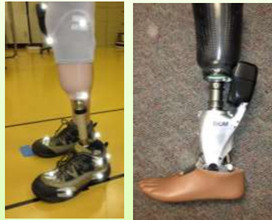
Investigations span from more simple passive devices (Left) to more complicated actively powered prostheses (Right).
