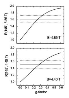
FIG. 2. The calculated double ratio  $R(145^0, B)$  vs the g factor, and the experimental double ratio for the 779–101 keV,  $0_2^+ \rightarrow 2_1^+ \rightarrow 0_1^+$  cascade, for the two values of the magnetic field used in this experiment.
