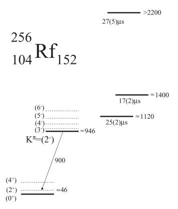
FIG. 3. Proposed decay scheme for <sup>256</sup>Rf. Energies are given in keV. Half-lives are written beneath each isomer.
