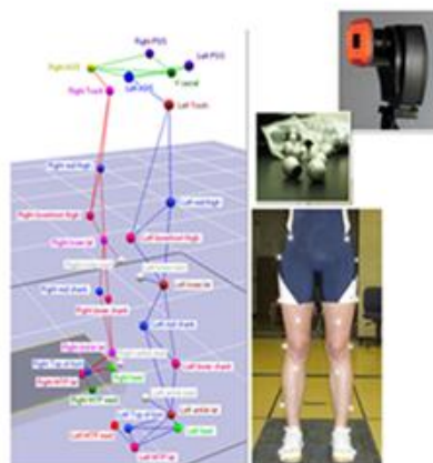
Figure 4. Lower limb marker set and a camera
