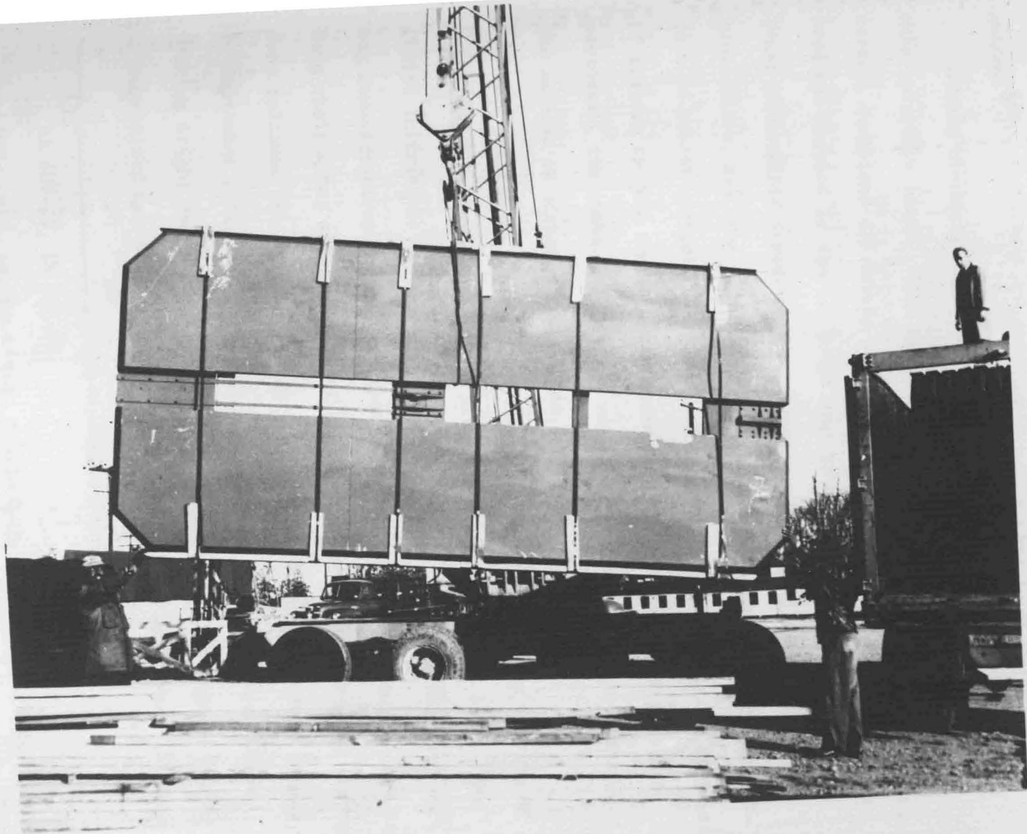
THE 18' PLATFORM BEING UNLOADED IN THIS VIEW WAS OF A TYPE USED FOR THE DROPPING OF A 9-TON BULLDOZER BY PARACHUTE
