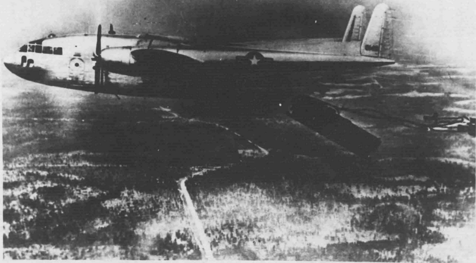
A 2½ ton truck just after leaving the cargo aircraft. The 2½ ton truck was not dropped by the Airborne Group during the first year and a half of training but future development plans called for rigging and dropping of the truck probably in the spring of 1953.
