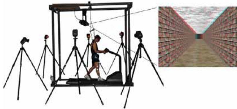
Fig. 1. Experimental set up consisting of the treadmill and the body weight support system and the six-camera motion capture system. The projector was located right behind and above the subject's head and three meters away from the screen to ensure a wide field of view for the subject. On the right side, the virtual reality (VR) environment is shown as it appeared to the subject without the red-blue stereo glasses. The use of a stereo graphics card (nVidia Corporation, Santa Clara, CA) renders not one but two separate images on the screen. On viewing them with the stereo glasses, the two scenes merge and there is a feeling of depth of the rendered scene.
