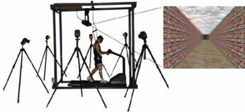
Fig. 1. Experimental set up consisting of the treadmill, the BWS, the VR and the eight-camera motion capture system (only six are shown in the figure). The projector was located right behind and above the subject's head and three meters away from the screen to ensure a wide field of view for the subject. On the right side, the virtual reality (VR) environment is shown as it appeared to the subject without the red-blue stereo glasses. The use of a stereo graphics card (nVidia Corporation, Santa Clara, CA) renders not one but two separate images on the screen. Viewing them with special glasses creates a feeling of depth of the rendered scene.
