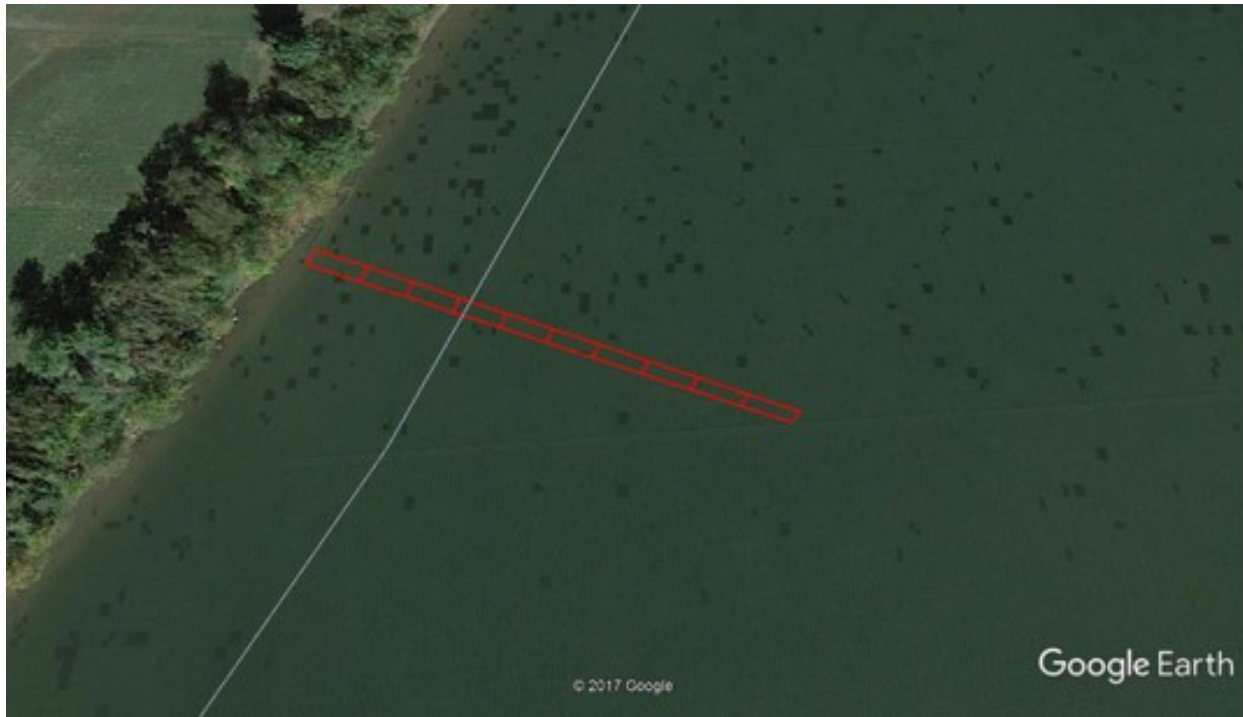
Figure 14. Typical 100 meter transect layout. Each cell (intersect) is 1X10m 2 (Source: Google Earth Pro).
