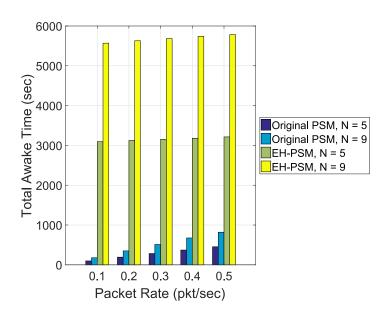
Figure 8. The performance of total active time period against packet rate and number of nodes.
