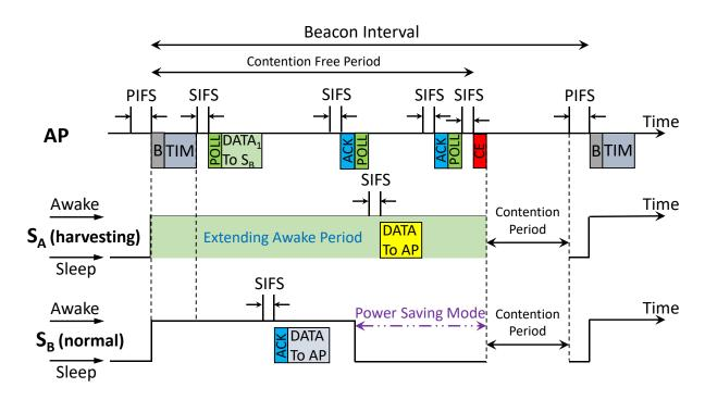
Figure 3. An example of node in energy harvesting mode extends awake period.
