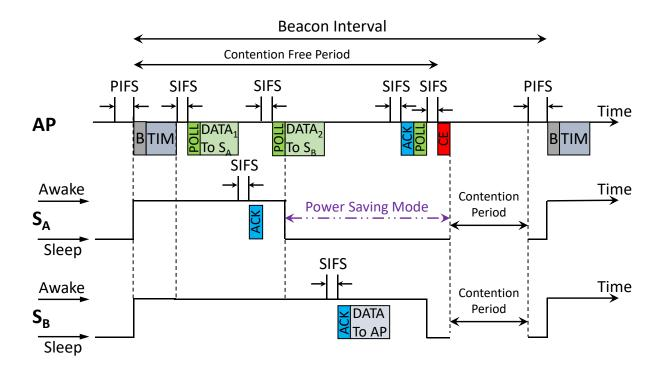
Figure 1. A snapshot of the power saving mechanism of IEEE 802.11.
