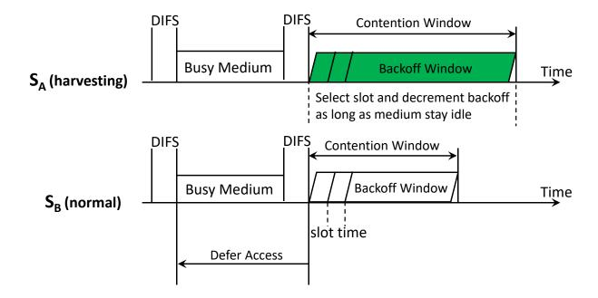
Figure 2. An example of longer contention window for a device in energy harvesting mode.
