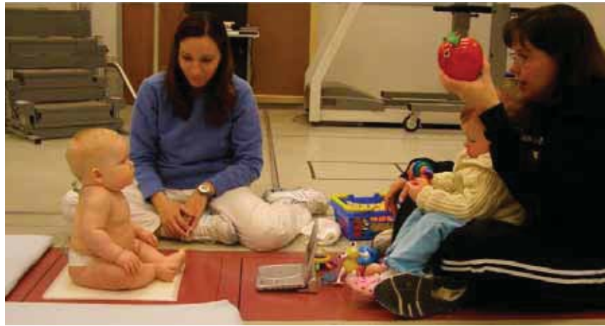
Figure 1 — Postural sway COP data were collected as an infant sits on a force plate. COP data were used to train the neural network.
