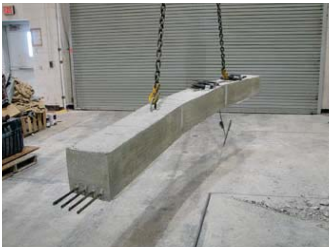
Figure 18. Two-point lifting points were installed at 3 ft from either end of the beam and lifted by a crane with a chain, which formed an angle of 75 degrees with the beam and the chain. The beam was lifted by a crane with an inclined chain. Note: 1 ft = 0.305 m.
