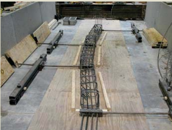
Figure 11. For the deviators and support layout, each deviator was attached to a 1-in.-diameter threaded rod. Note: 1 in. = 25.4 mm.
