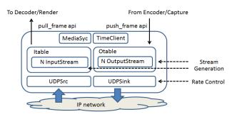
Figure 6: Streaming System for scheduling and prioritization
