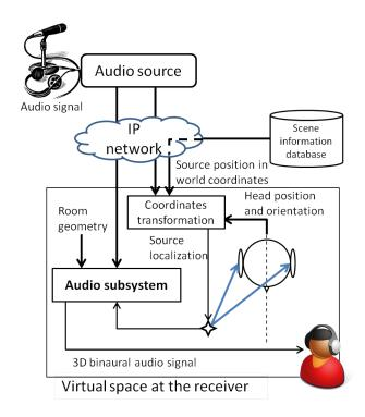
Figure 1: Overall communication architecture for the virtual scene composition and rendering.
