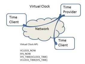
Figure 4: Global Timestamp distribution for virtual clock synchronization with local to global conversion API
