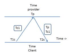
Figure 5: Sequence diagram for sync messages for virtual clock synchronization
