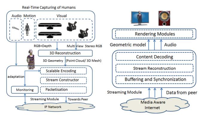
Figure 3: Source location (left) and destination location (right) of the media pipeline.
