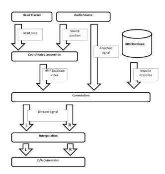
Figure 2: The workflow diagram of the audio subsystem.
