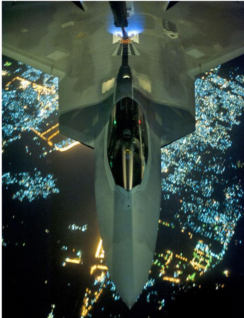
Figure 1. Midair refueling of an F-22 Raptor. Photo credit: Tech. Sgt. Russ Scalf, U.S Air Force
