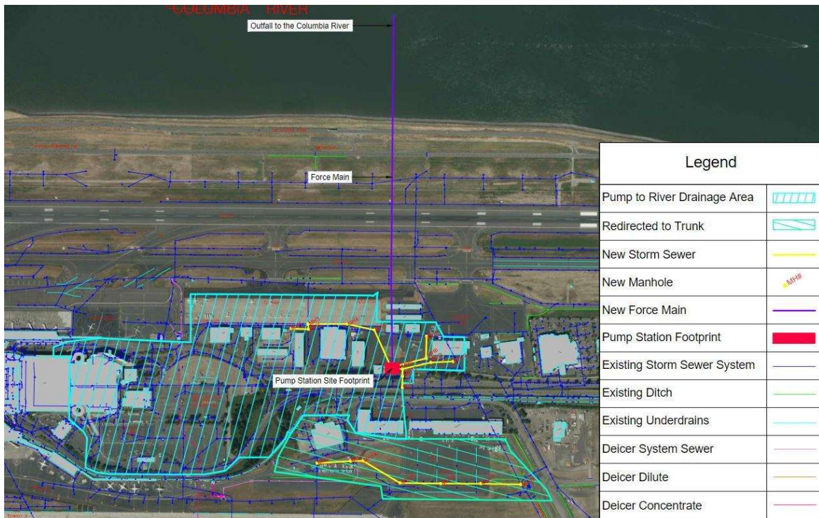
Figure 15. Area of Basin 7 to be directed to the pump station (Gresham Smith, 2014).
