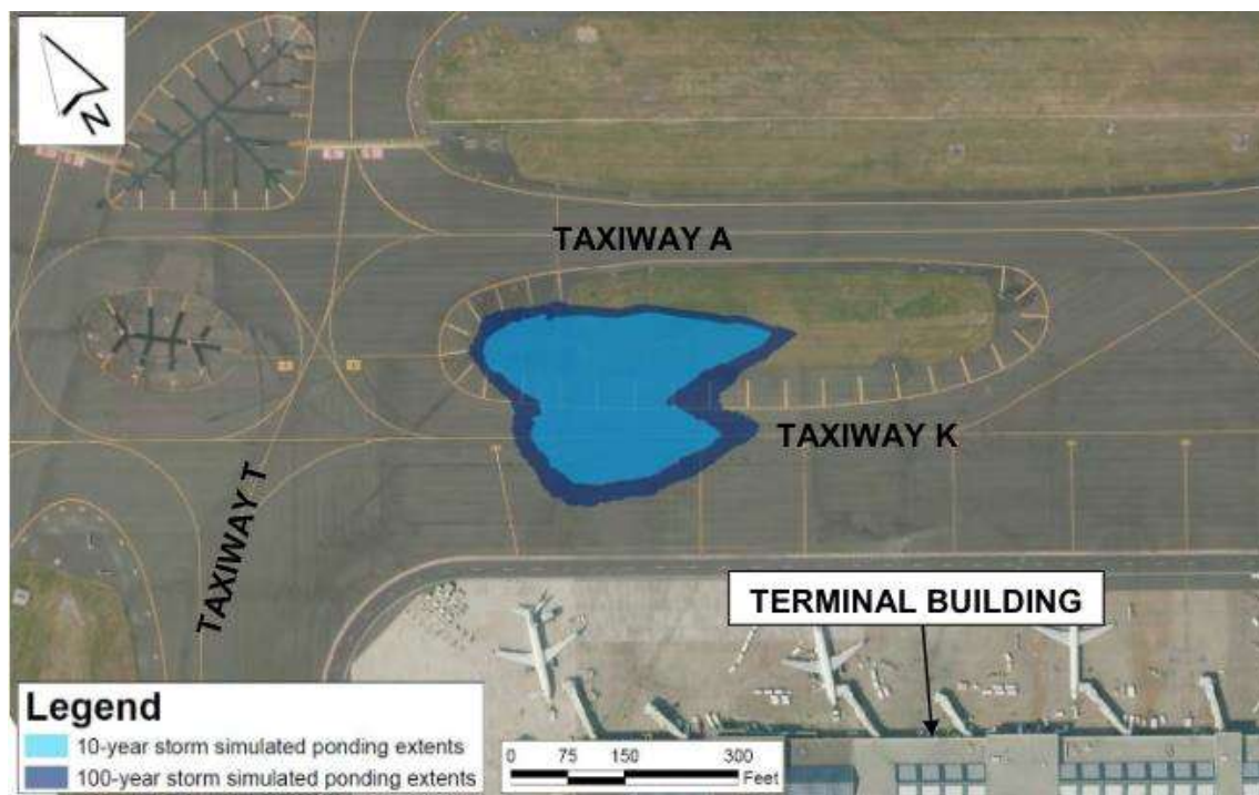
Figure 7. Ponding issues located at Taxiway A and K within Basin 7 (Port of Portland, 2015).
