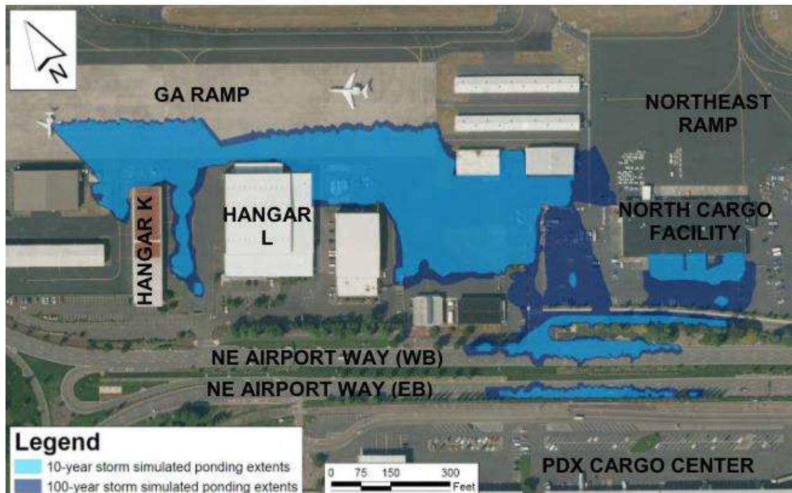
Figure 6. Ponding issues located at Hangar K, Hangar L, the North Cargo Facility, NE Airport Way, and the Atlantic Aviation Facility within Basin 7 (Port of Portland, 2015).
