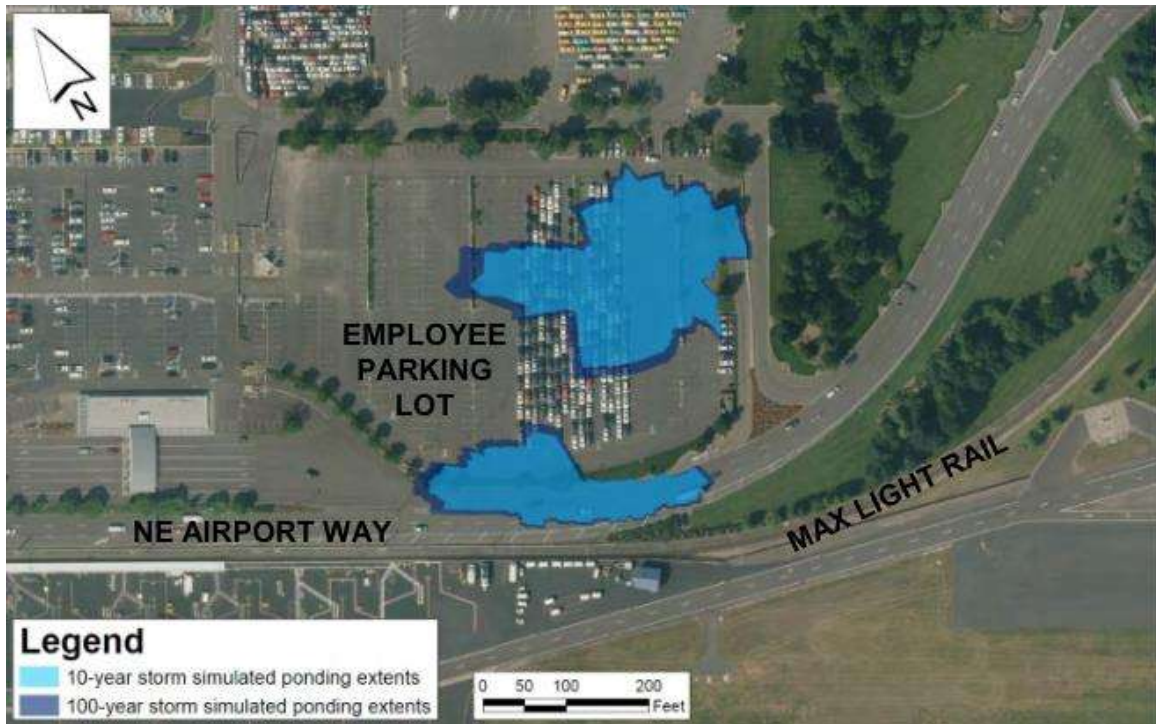
Figure 5. Ponding issues located at the employee parking lot within Basin 7 (Port of Portland, 2015).
