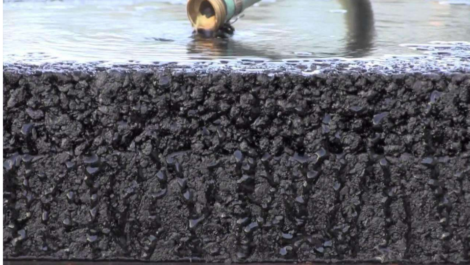
Figure 12. Visual representation of pervious pavement (Auburn University, 2015).
