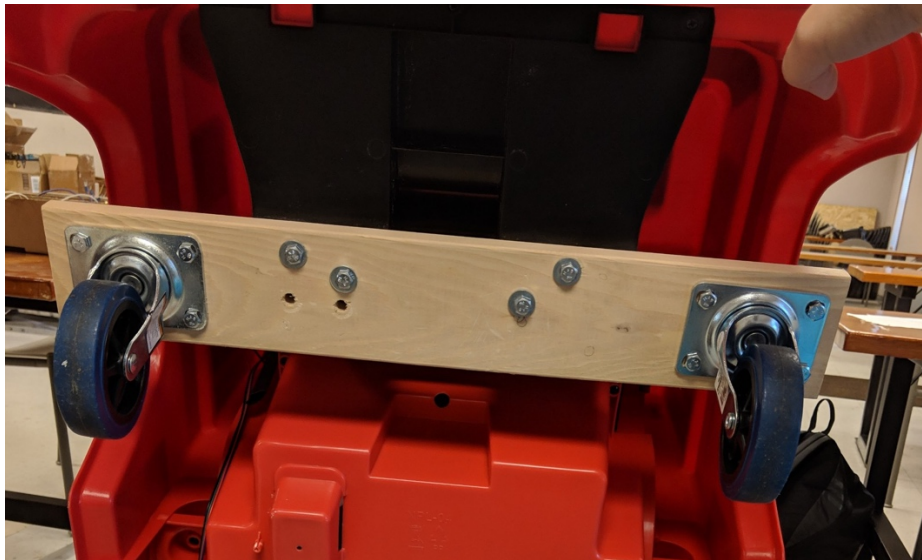
Figure 1: Swivel wheel system for previous Go Baby Go car design
