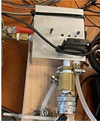
Figure 18: Valve Delay Testing Set-up
