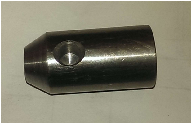
Figure 18: The locking bolt with hole for the pin
