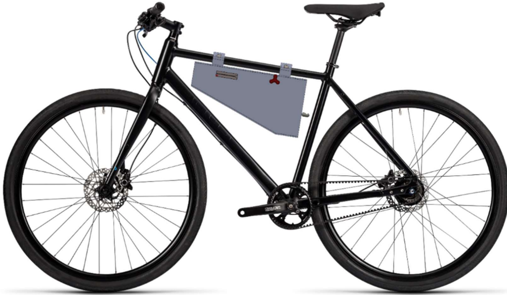
Figure 3. Using the inner triangle of the bike for the positioning of the lock the BorrowBike lock can utilize the most space.
