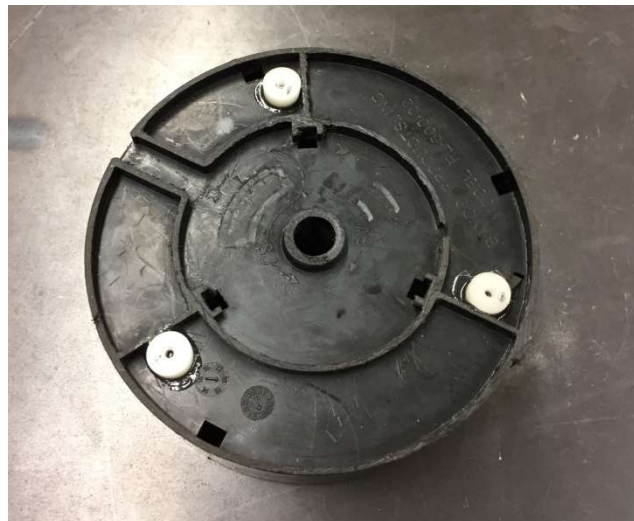
Figure 10. The cut side of the drum with nylon blanks for machine screws.
