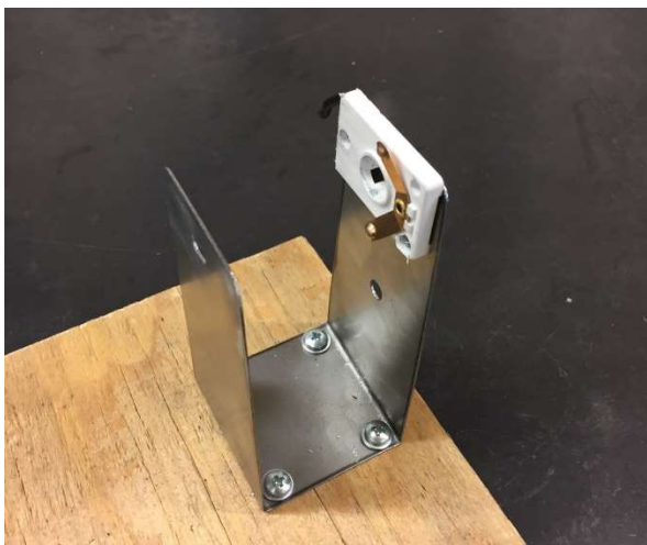
Figure 15. The sheet metal replacement spool mount and brushes recycled from the cable reel.
