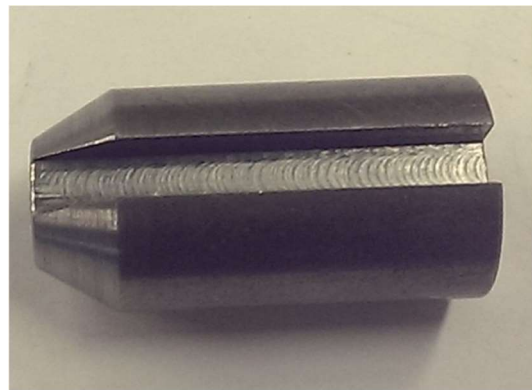
Figure 17. The slot on the underside of the locking bolt.
