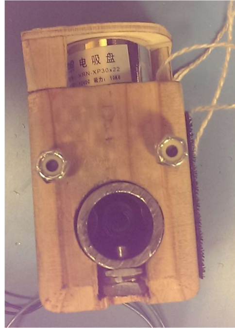
Figure 20. The finished lock assembly.
