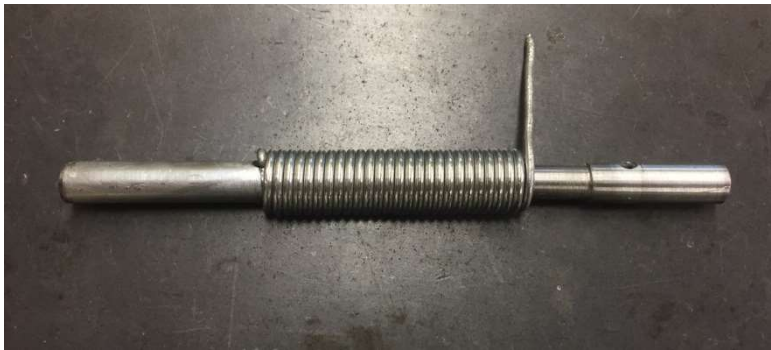
Figure 1. The prototype torsion spring and mandrel assembly. Figure 2. Wooden spool mockup.
