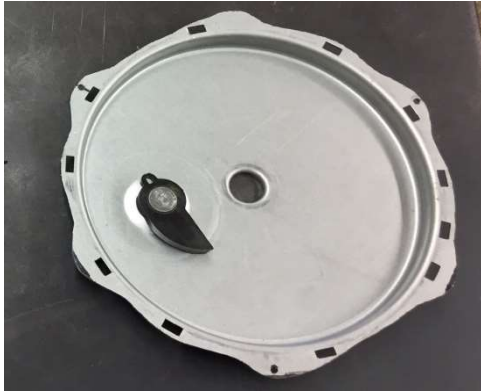
Figure 11. The ratchet end-plate after removal of most of the flange.
