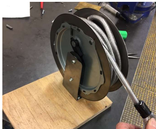
Figure 16. The finished retractable cable spool and ratchet system.
