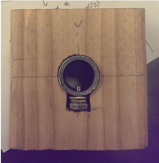
Figure 19. The lock receiver press fit into wood.
