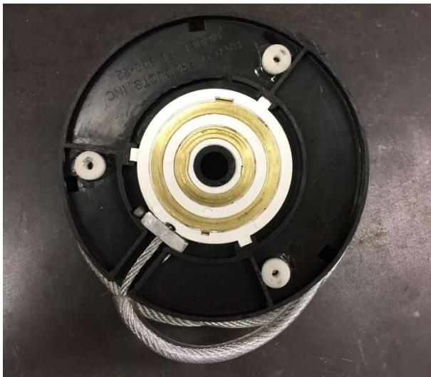
Figure 13. Cable attachment mechanism and the brush contacts recycled from the cable reel.
