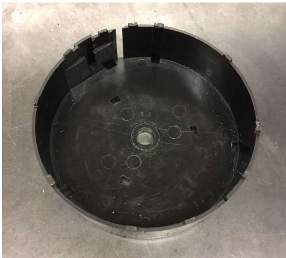
Figure 9. The spool drum after being cut to 2.1in thick. Cut side opposite of shown.
