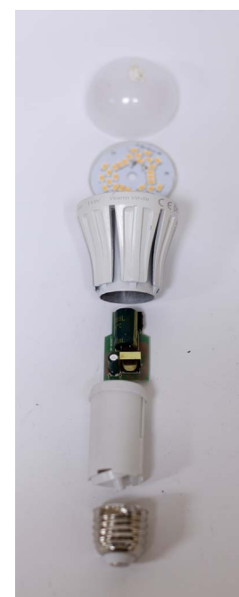
Figure 14. P03 product with removable fasteners and limited adhesives.
