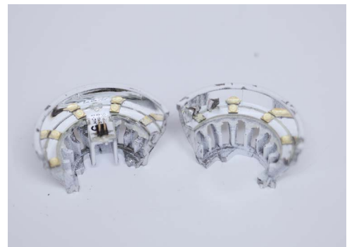
Figure 10. P02 product disassembly with heat exchanger in two parts. The sections required a dremel tool for separation.
