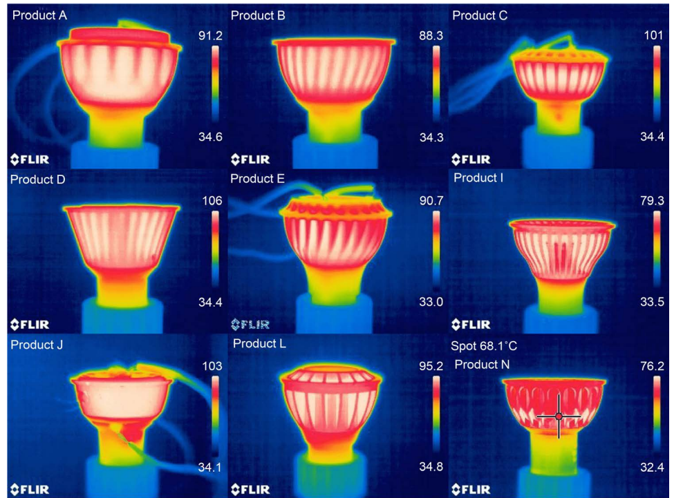
Figure 1. Infrared camera images of each product used for orientation and thermocouple placement.
