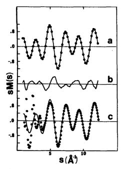
FIG. 1. Reduced intensity curves: (a) Pure CCl<sub>4</sub>. Points, experimental (0.12 bar). Solid line, theoretical monomer. (b) Systematic difference between the experimental and theoretical curves multiplied by 8 (see the text). (c) Points, experimental data for CCl<sub>4</sub> (0.12 bar) with neon carrier (1.3 bar). Solid trace, theoretical curve for CCl<sub>4</sub> monomer. Note the strong cluster signal at small scattering angle.
