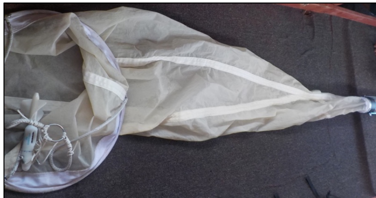
Figure 5. Photograph of plankton net (150 \mu\text{m} ) used for micro-plastic sampling. Photograph taken by CJ O'Brien.
