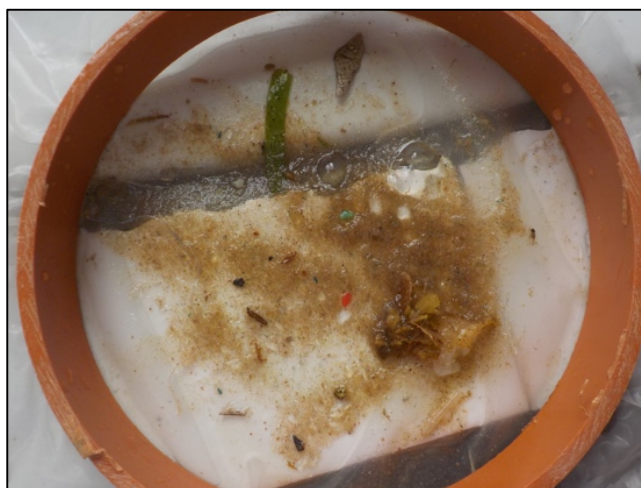
Figure 6. Photograph of sieve (100 \mu m) used for plankton and micro-plastic separation. Photograph taken by CJ O'Brien.
